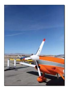
The diesel RV-9 sports a three-blade MT prop. The Van's Aircraft factory RV-9A, in the background, features a Lycoming O-320 and a two-blade Hartzell constantspeed prop.
