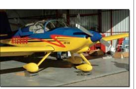
To be sure about weights, the Van's factory RV-9A is placed on electronic scales; the Wilksch was weighed immediately after. The diesel aircraft is actually 57 pounds lighter overall.
