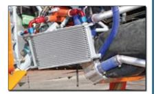
The oil cooler is fed air from a sidemounted NACA duct.
