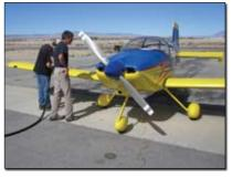
At the end of each flight, both aircraft were refueled and their consumption compared. In each case, the Wilksch consumed fewer gallons of fuel than the Lycoming.
