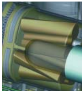
The old supercharger internals feature a complex twisted shape difficult and costly to machine – they also weigh rather a lot
