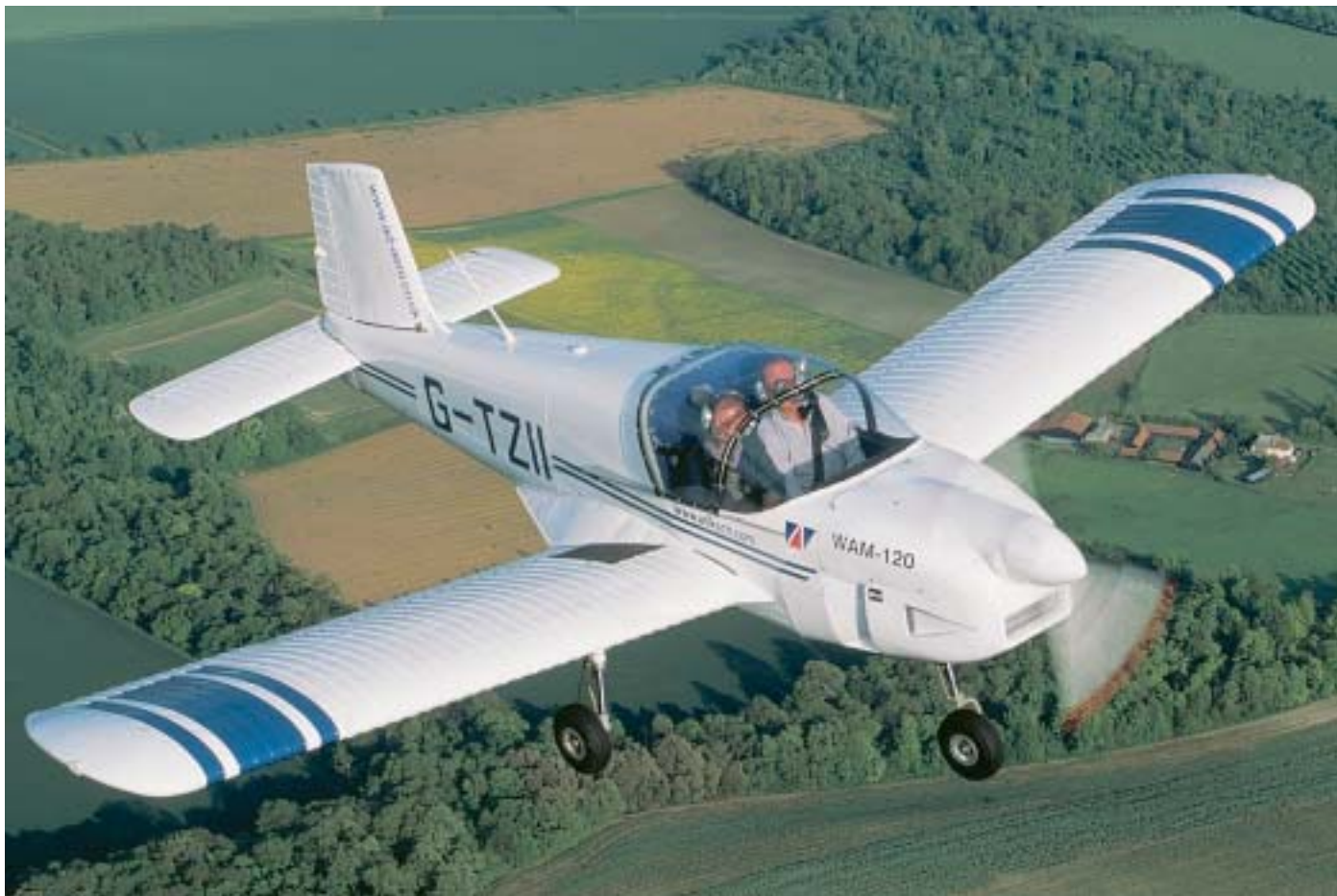
The Thorp is surprisingly small – 577kg MAUW – and although empty weight is 14kg more than original, 20kg less fuel is required to achieve same range
