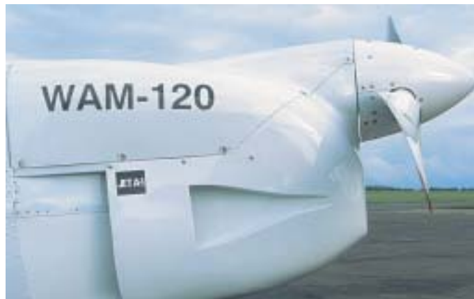
Side NACA duct feeds the oil cooler. WAM makes no apologies for the boxy but functional cowl – future installations will probably feature elliptical inlet
