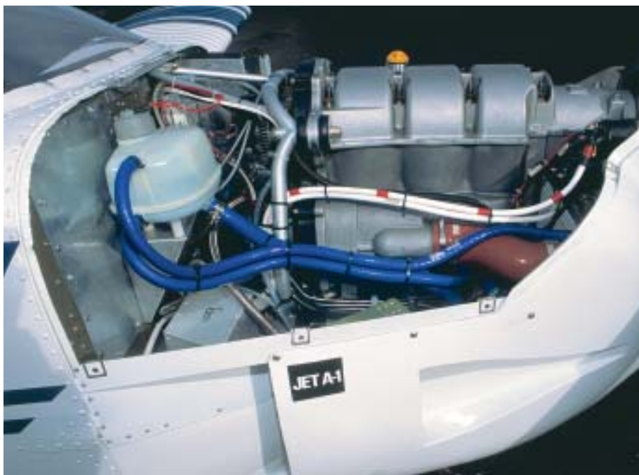
Neat installation, allowing plenty of room. The coolant bottle cap sensor is a pre-flight check item
