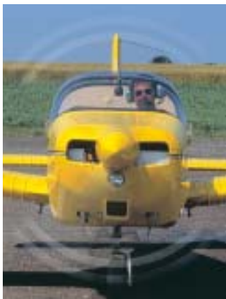
The O-200 engine installation actually has larger inlet – 500cm 2 ...
