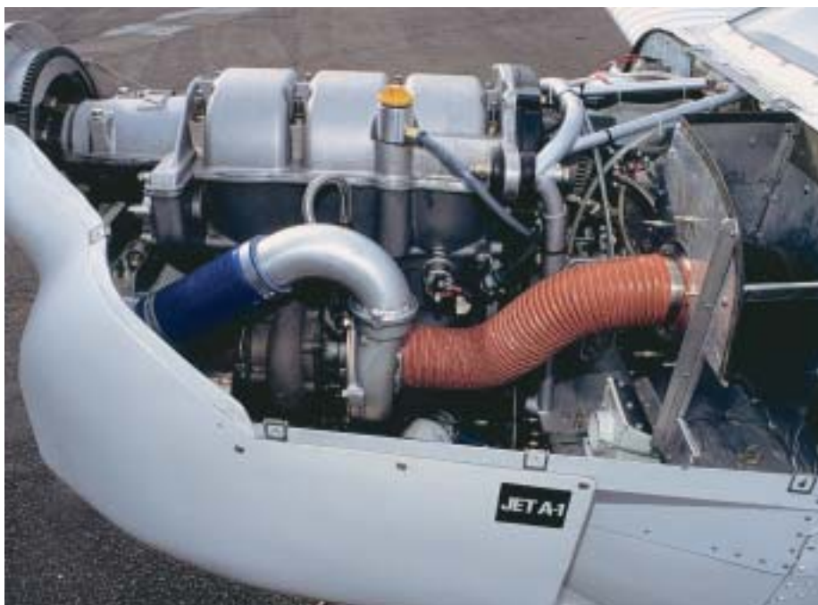
Oiled foam conical air filter is a WAM item – scat hose will be replaced with a moulded silicon version
