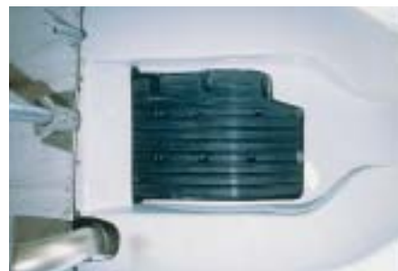
The exposed oil sump helps with cooling – flight trials are continuing to assess its effectiveness
