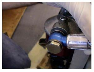
16) Push and twist hose end into lift pump until fully seated. Re-fit retaining clip and torque filter end, 25-30 NM.
