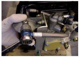
2) Remove retaining clip from the lift pump end using a screwdriver and fingers. CAUTION: Do not let this clip spring off. Gently twist and pull the fuel line out of the lift pump.
