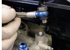
4) Support the fuel filter with your hand and undo the banjo bolt, but only enough to free the hose.
