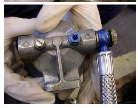
Fit to fuel filter (pressure outlet end).
