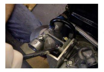
5) Unfasten the fuel filter retaining nuts with a 10mm spanner.
