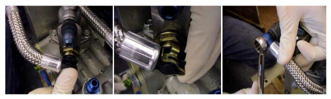
17) Remove fuel return fitting and discard washer. Fit new washer and torque to 25-30 NM.
