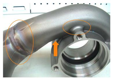
Pay special attention to the areas highlighted, such as the welded joint between the manifold branch and the turbo scroll, the radii where the attachment bosses blend into the tube and the "Vee" ,indicated by the arrow, where the scroll meets the tube.
