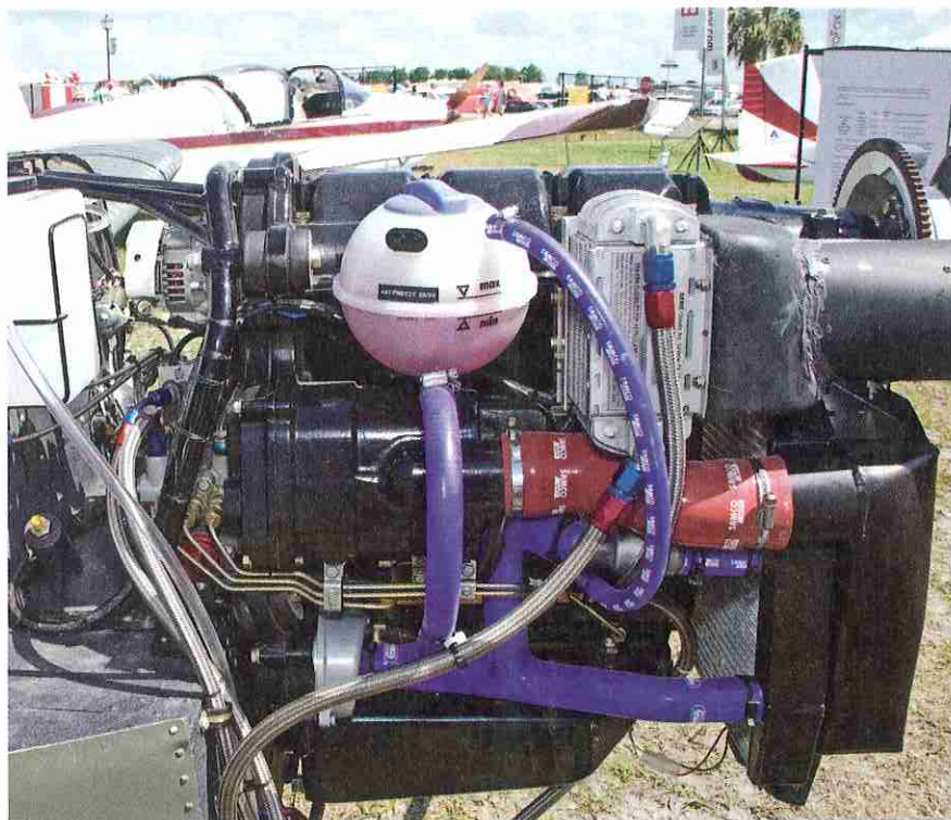
The right side of the engine, showing from left to right, the smoke oil tank, coolant reservoir, the oil cooler (which is low, front and center in the production model), and the radiator stacked behind the intercooler. The intercooler is a split system - left and right - tucked completely inside the cowl on the production model.
