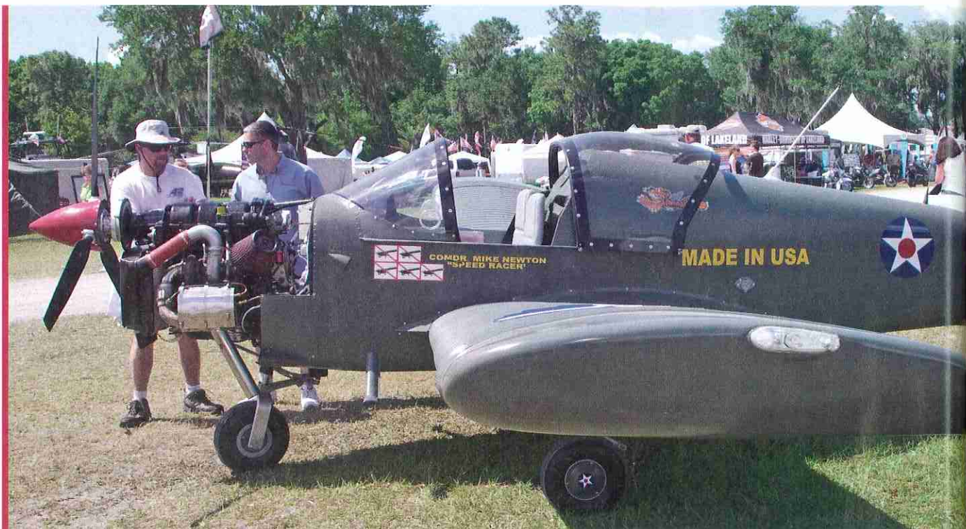
The intake air filter and exhaust muffler can be seen here. The production model eliminates the muffler and is quieter. The production model also puts the intercooler, oil cooler inside the cowl, with the radiator hung on the belly.
